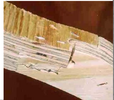
5-layer, 7-ply (3 parallel center plies)
